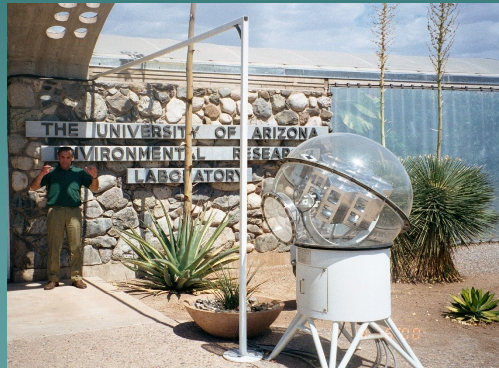
Figure 2. The optical waveguide (OW) solar plant lighting system for simultaneous PAR transmission and PV power generation.
