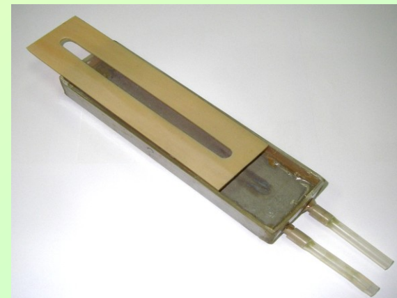
Vessel for plant growing equipped with porous metal-ceramic membrane
