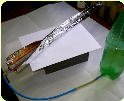
Porous metal-ceramic tube with fibrous ion-exchange artificial soil
