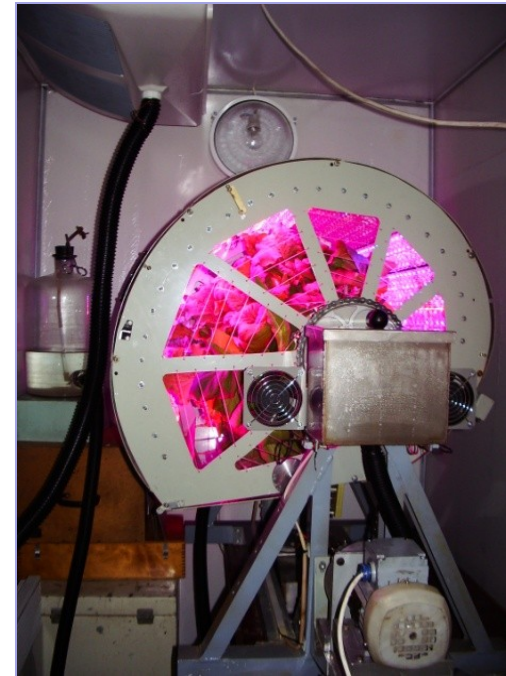
Ground modal of the space conveyer plant growth facility “Phytocycle-LED”, arranged in the climatic chamber “POLAIR”
